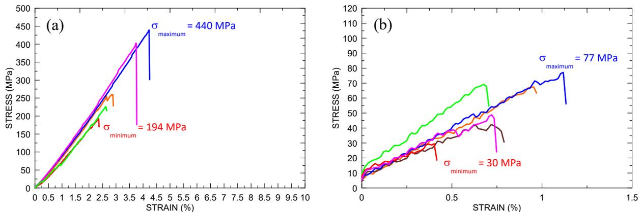
Fig. 4. Stress vs. strain for biomorphic SiC derived from (a) tornillo wood and (b) bolaina wood obtained in uniaxial compression and at room temperature
