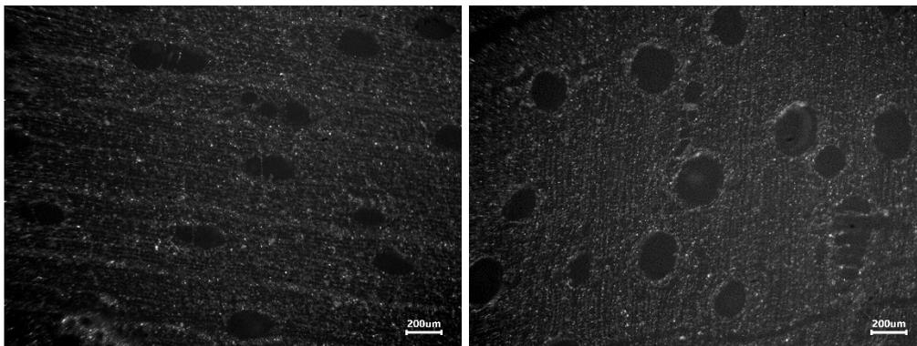
Fig. 2: Micrographs of the carbon cross section obtained by optical microscopy from samples (a) bolaina and (b) tornillo
