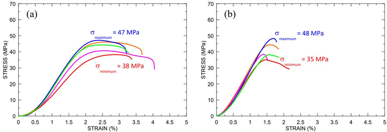
Fig. 3: Stress vs. strain for (a) tornillo wood and (b) bolaina wood tested at constant compression rate and at room temperature
