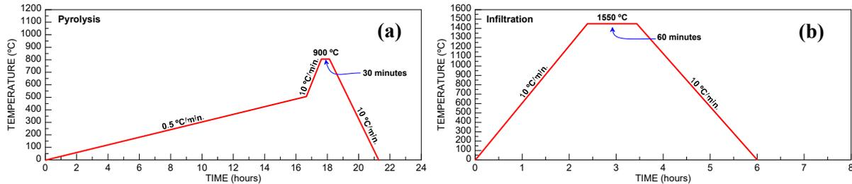
Fig. 1: Thermal profiles for the processes of (a) pyrolysis and (b) reactive infiltration.
