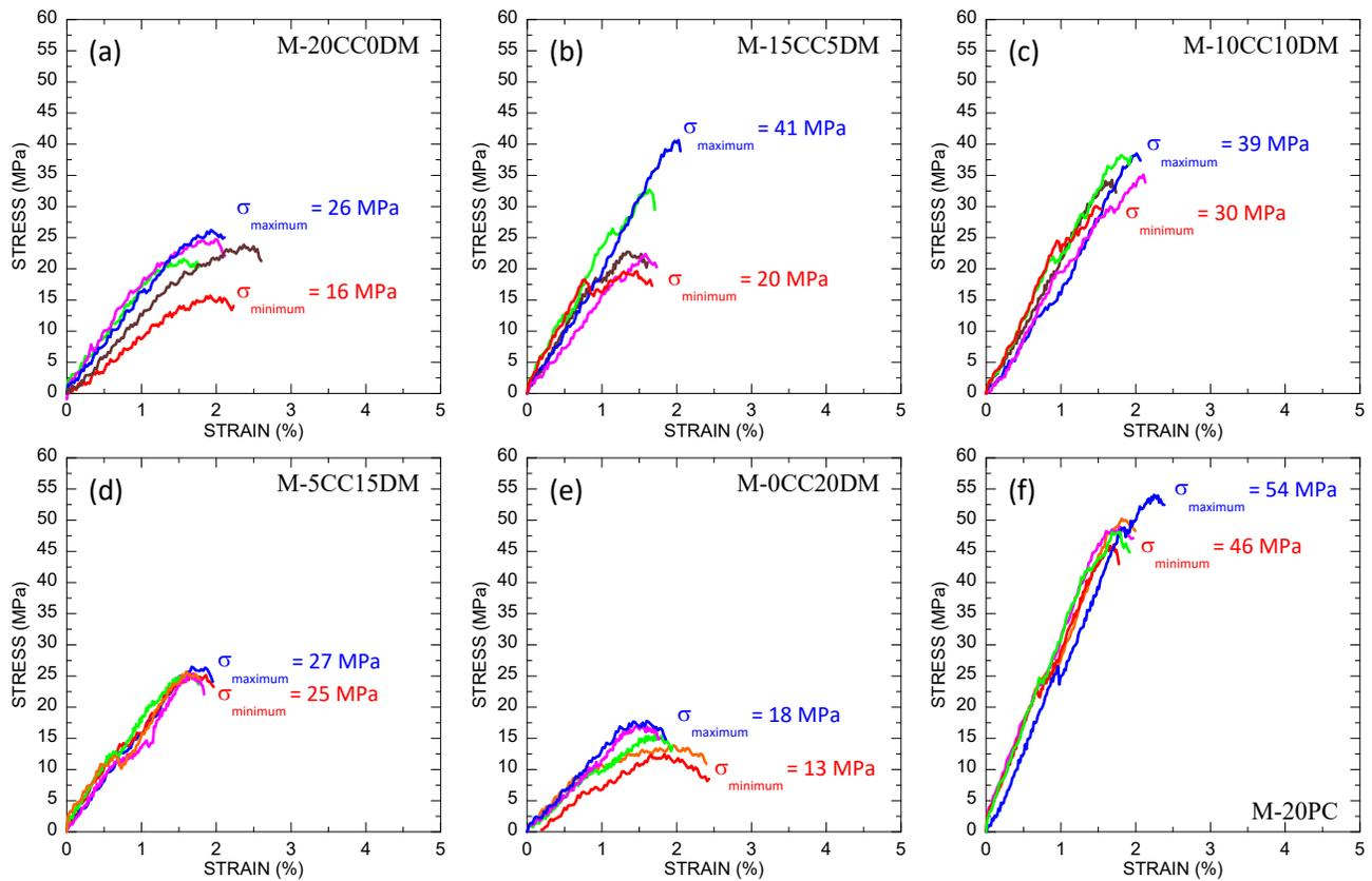
Fig.2: Stress vs. strain curves for the six types of mortars studied
