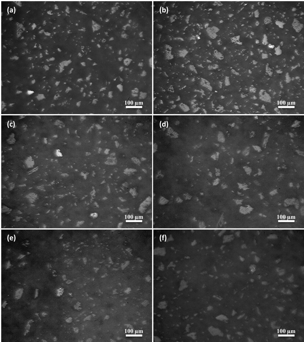
Fig. 1: Light microscopy micrographs of geopolymeric (a-e) and conventional Portland cement mortars (f)
