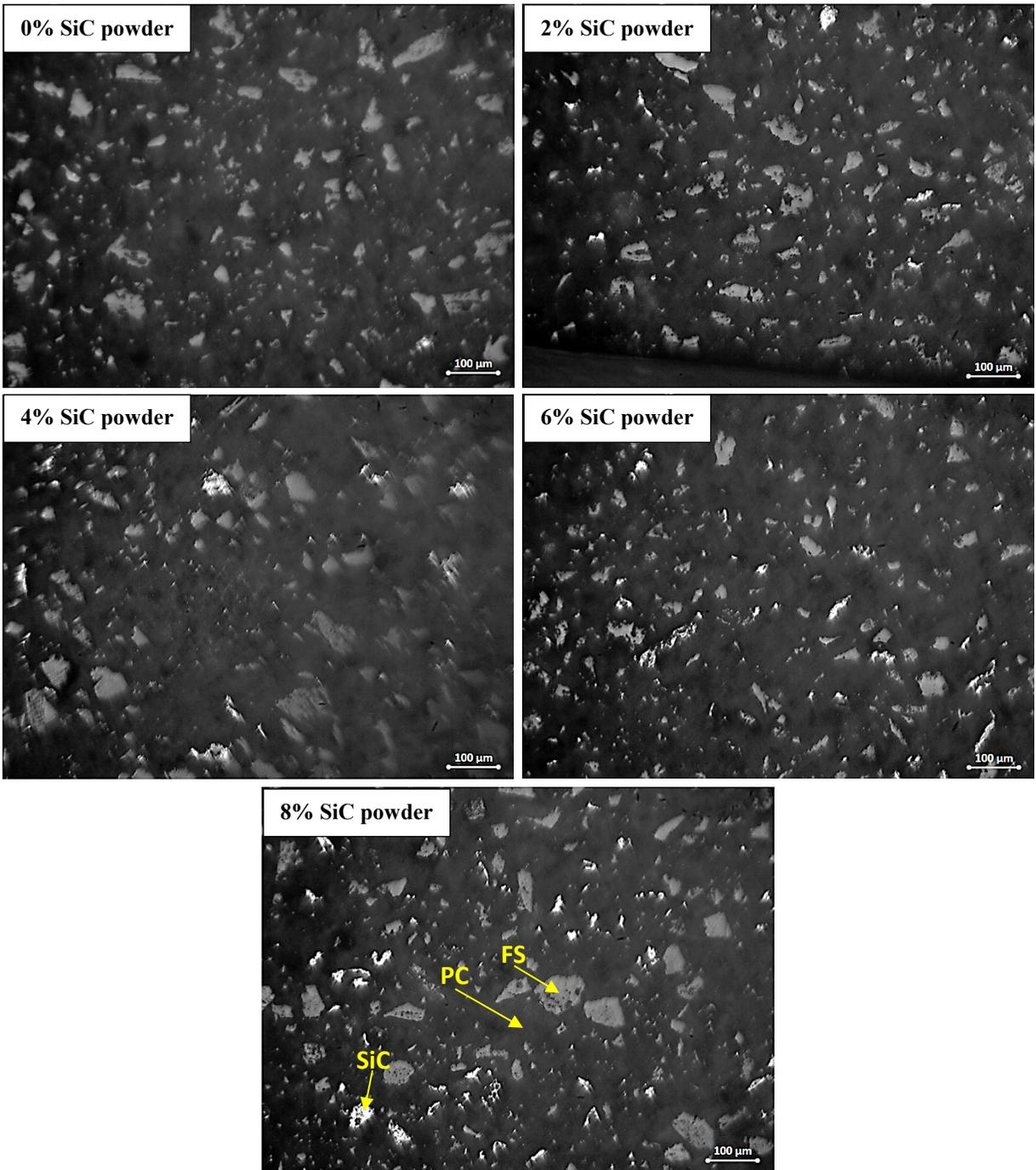
Fig. 2: Optical microscopy micrographs of cement Portland mortars with various percentages of SiC powder added.
