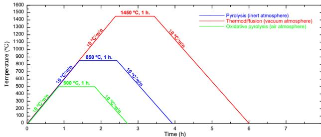
Fig. 1: Thermal profiles for inert pyrolysis (blue line), thermodiffusion (red line) and oxidative pyrolysis (green line) processes
