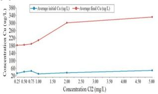
Fig. 6. Copper corrosion rate versus residual chlorine concentration
