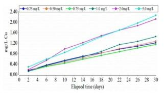
Fig. 7. Impact of residual chlorine on the cumulative concentration of copper released during the static immersion test.
