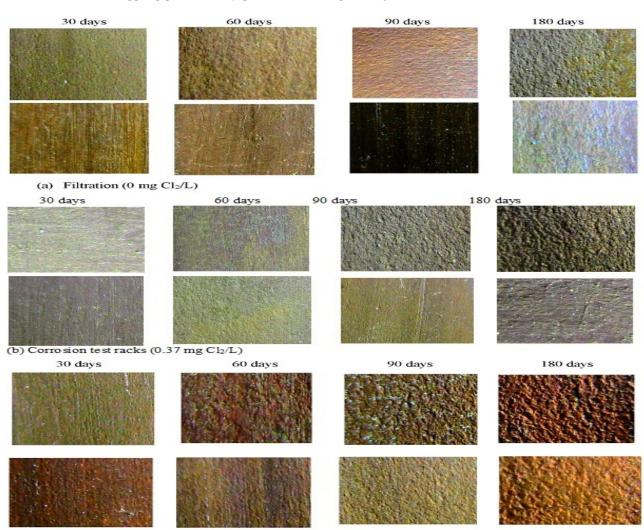
(c) Storage tank (0.85 mg Cl<sub>2</sub>/L)
