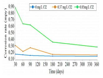
Fig. 5. Copper corrosion rate versus exposure time
