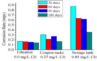
Fig. 4. Copper corrosion rate versus free chlorine concentration
