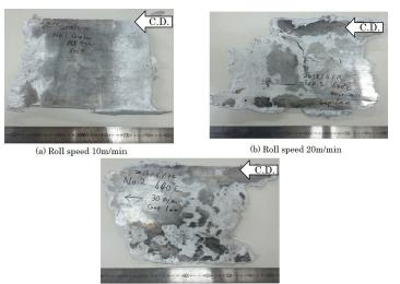
(c) Roll speed 30m/min Figure 5: Produced strips.
