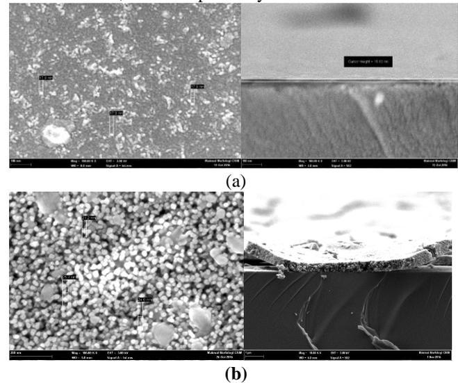
Fig. 1. Nanocrystalline thin film produced at the heating temperature 500 °C using (a) spin coating (b) chemical bath deposition method
