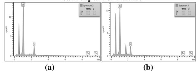
Fig. 2. EDX spectra (a) spin coating method (b) chemical bath deposition method
