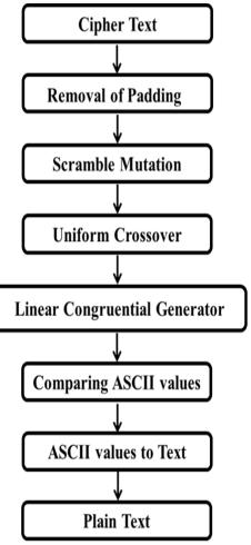
Fig. 5. Block Diagram of Decryption Process
