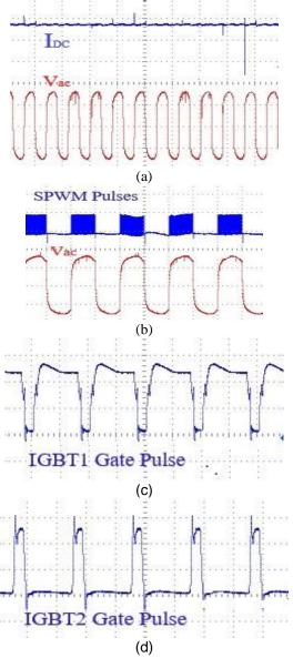
Fig. 8. Experimental outcomes of the projected 1-¢ bridge inverter: (a) Incoming DC current with output side AC Voltage (b) SPWM Pulses with respect to output voltage (c) Gate Pulse for IGBT1 of Buck-Boost converter (d) Gate Pulse for IGBT2 of Buck-Boost converter
