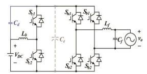
Fig. 3. Bridge inverter built on buck-boost convertor.
