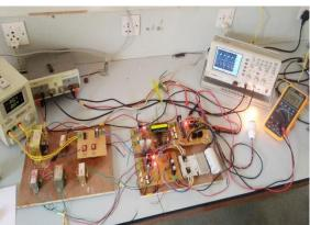
Fig. 6. Hardware of the projected 1-φ bridge inverter.
