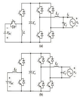
Fig.1. 1-φ bridge type inverter with: (a) buck-boost convertor; (b) boost convertor.
