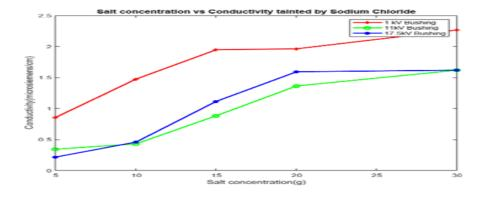
Fig. 2. Salt concentration and conductivity tainted by sodium chloride
