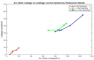
Fig. 6. Arc flash voltage and leakage current tainted by potassium nitrate
