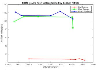
Fig. 10. ESDD and arc flash voltage tainted by sodium nitrate
