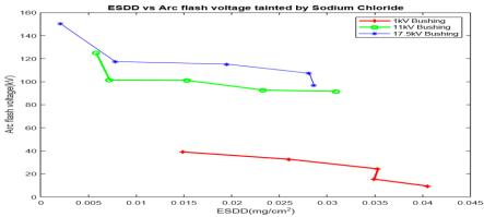
Fig. 4. ESDD and arc flash voltage tainted by sodium chloride
