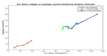
Figure. 3. Arc flash voltage and leakage current tainted by sodium chloride
