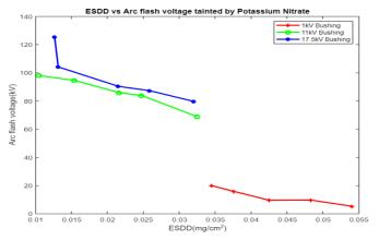
Fig. 7. ESDD and arc flash voltage tainted by potassium nitrate
