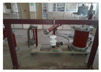
Fig. 1. Tentative setup for pollution testing
