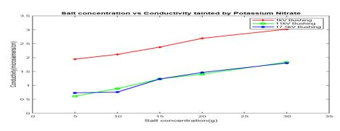
Fig. 5. Salt concentration and conductivity tainted by potassium nitrate
