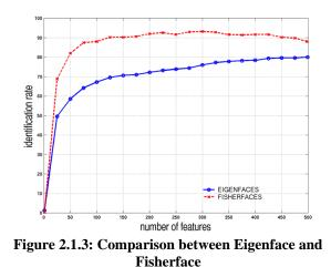
As the below figure clearly tells that Fisherfaces algorithm is better than Eigen faces algorithm.
