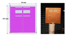
Fig. 3: (A) Proposed antenna with dimensions (B) Manufactured antenna
