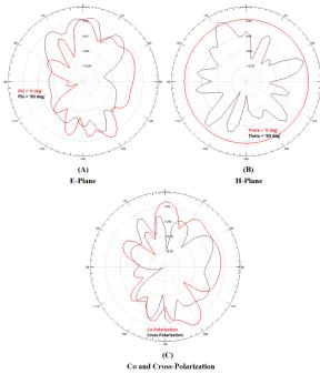
Fig. 5: Simulated Radiation Patterns at resonant frequency of 10.5 GHz - (A) E-Plane, (B) H-Plane, (C) Co and Cross-polarization
