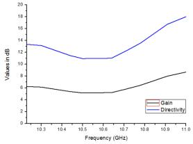
Fig. 7: Simulated values of directivity vs. gain of the converged antenna design
