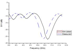
Fig. 4: Plot of measured vs. simulated return losses (S11) of the converged antenna design.
