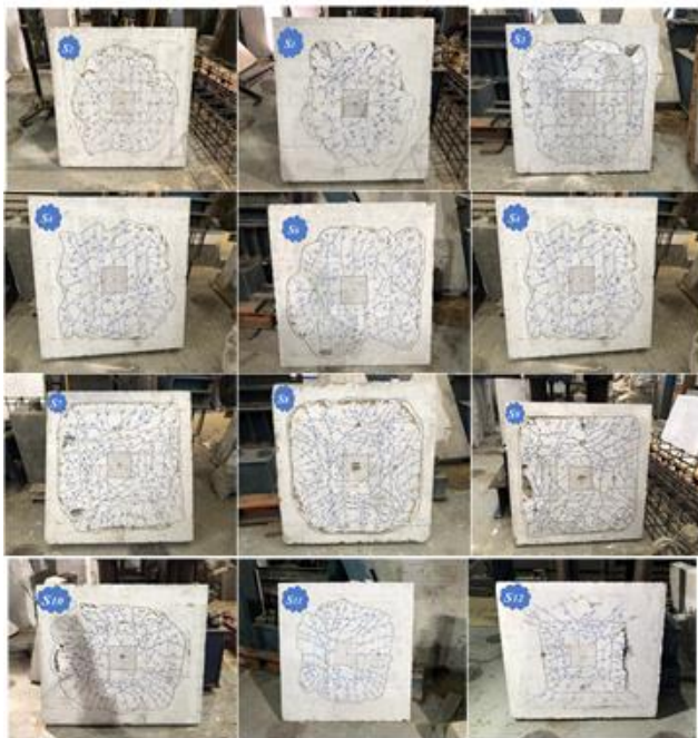
Fig.10. Cracking Patterns of Specimens (S1 to S12)
