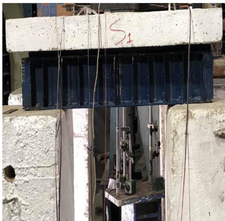
Fig.9. Location of the Three LVDTs
