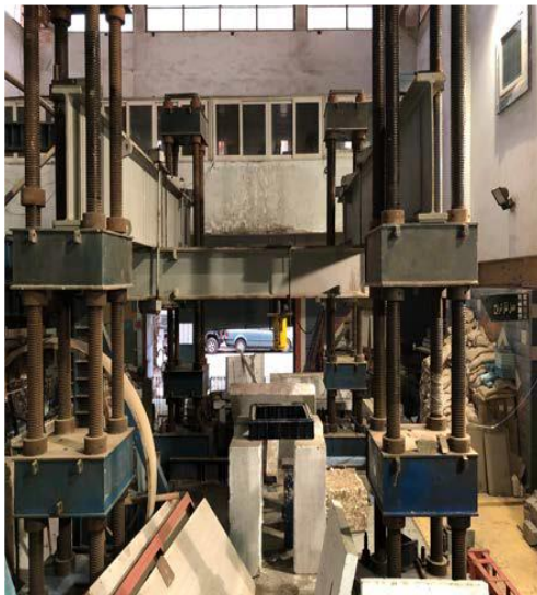
Fig.8. Load Set up for Test Specimens
