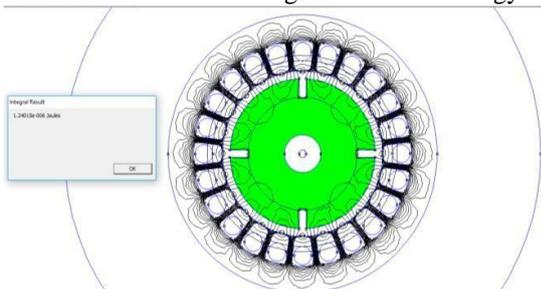
Fig 19. Magnetic field co-energy calculation
