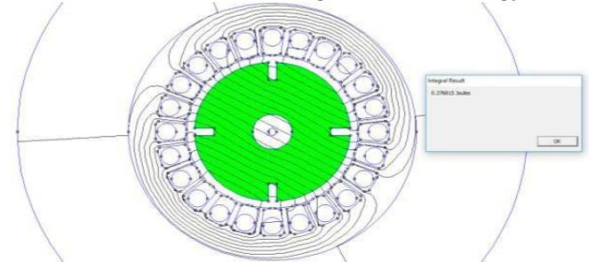
**Fig 29. Magnetic field co-energy calculation**
