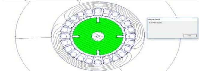
**Fig. 30. Magnetic field energy calculation**
