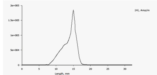
Fig 21. Plot of Magnitude of Magnetic field intensity v/s length of selected lines
