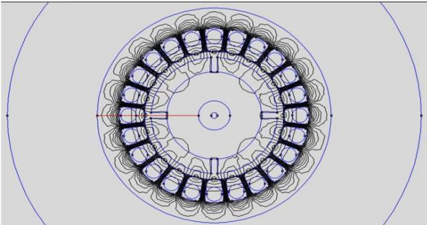
Fig 17. Grey Scale representation of Flux density field
