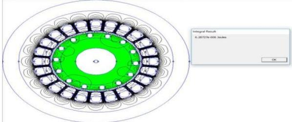
Fig 9. Calculation of Magnetic field energy
