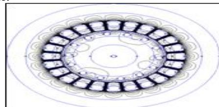
**Fig 4.Generated flux lines**
