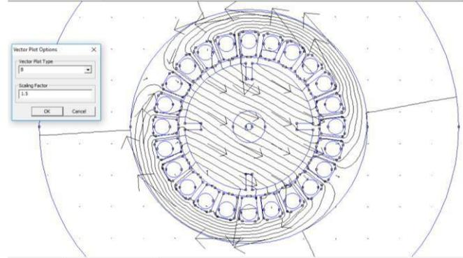
**Fig. 28. Vector direction of Magnetic field**
