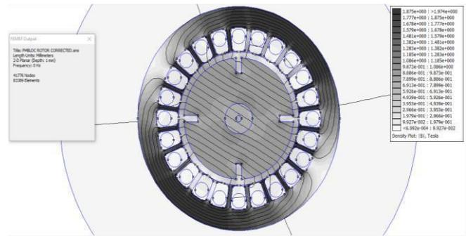
**Fig. 27 Grey scale representation for flux density distribution**
