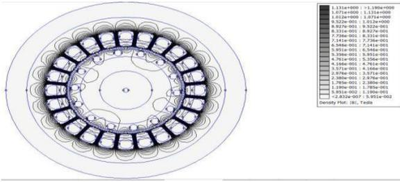
Fig 7. Grey scaling of flux density
