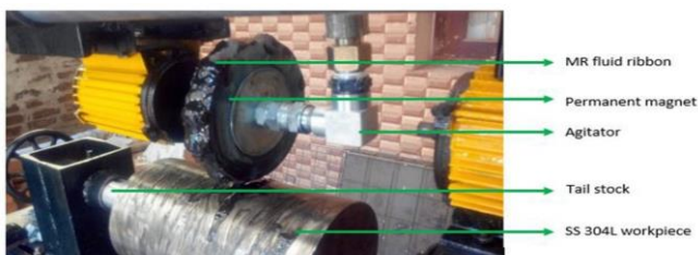
Figure 1. MR fluid cylindrical surface machining of AISI 304L stainless steel
