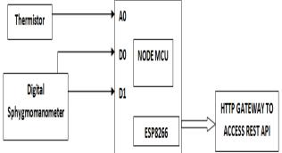
Fig.3. Stage 1 Flow Diagram of Proposed model
