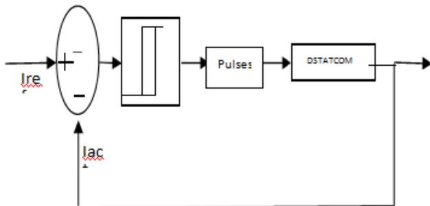
Fig.2. block diagram of hysteresis current control
