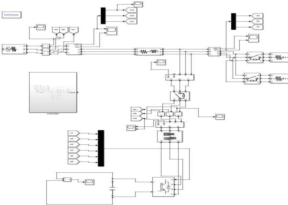
**Fig.4. Simulation model with D-STATCOM**
