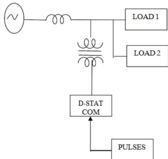
**Fig.1. Block diagram of D-STATCOM**
