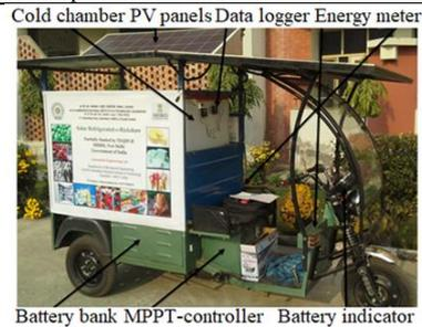
**Fig. 1. Example setup (a) block diagram (b) of SAREV.**
