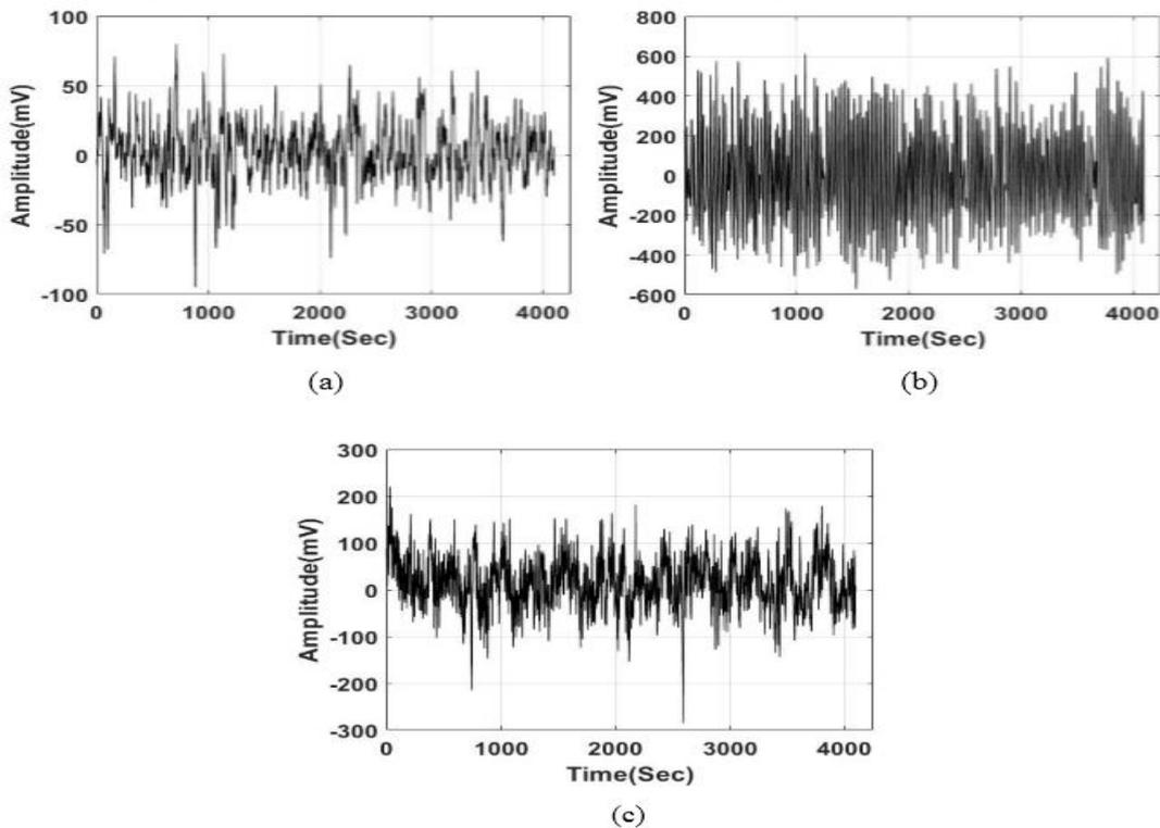
**Figure 3. BU EEG database; a) Ictal signal, b) Interictal signal, and c) Normal signal**
