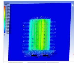
Fig.8: Temperature distribution on plane when hole diameter is 2 mm
