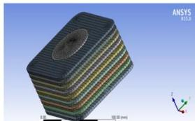
Fig.5: IC engine and cylinder meshed part without holes on fins
