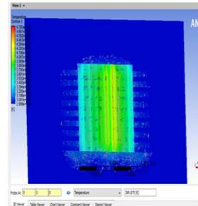
Fig.10: Temperature distribution on plane when hole diameter is 3 mm
