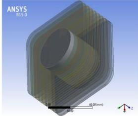
Fig.1: 3D geometry of IC engine cylinder and fins without holes on fins
