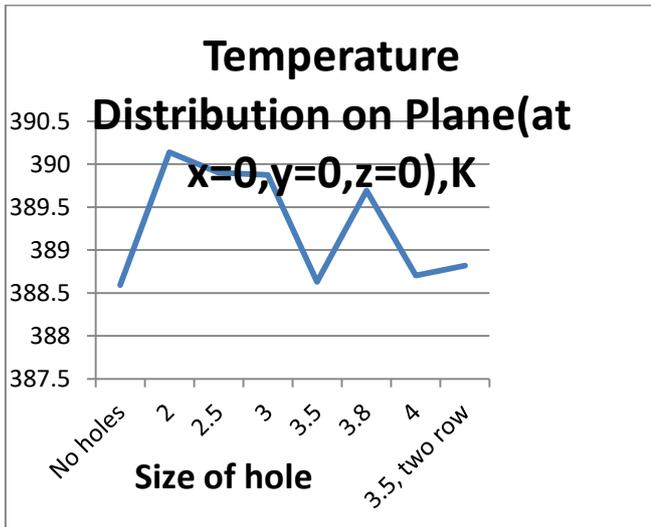
**Fig.15: Comparison of temperature between different hole diameters**
