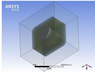
Fig.2: 3D geometry of IC engine and enclosure without holes on fins
