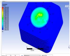
Fig.14: Temperature distribution on plane when two rows of hole with 3.5mm hole diameter
