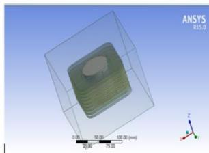
Fig.4: 3D geometry of IC engine and enclosure with holes on fins
