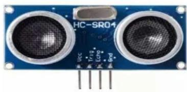
Fig. 3. Ultrasonic sensor
