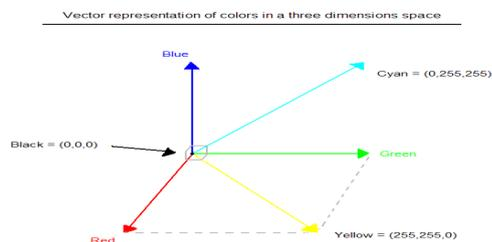
Fig. 2. Vector representation in Open CV
