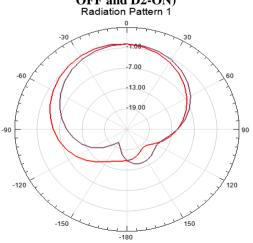
Fig.24 Proposed reconfigurable antenna Radiation pattern 2.2GHz (Diodes D1-OFF and D2- ON)
