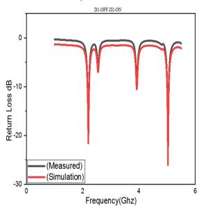
Fig.23 Proposed reconfigurable antenna return loss Simulation and Measured at 2.2,5.3 GHz (Diodes D1-OFF and D2-ON)
