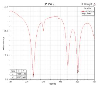
Fig.13 Proposed reconfigurable antennaVSWR 2.3 and 4.99GHz (Both the diode D1, D2 turns ON) • Two diodes D1,D2-OFF
