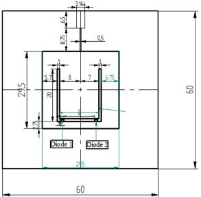
Fig. 7 Proposed Reconfigurable Antenna
