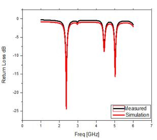
Fig.10 Proposed reconfigurable antenna return loss Simulation and Measured at 2.3,4.99GHz ( Both the diode D1,D2 turns ON)
