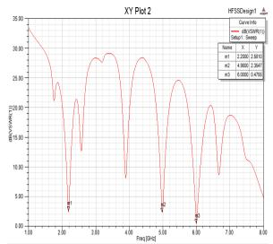
Fig.22 Proposed reconfigurable antennaVSWR 2.2, 4.98, 6GHz (D1-ON, D2- OFF) • Diode D1-OFF,D2-ON
