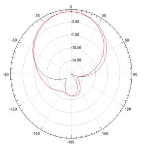
Fig.11 Proposed Reconfigurable Antenna Radiation Pattern 2.3 GHz (Both the diode D1, D2 turns ON) Radiation Pattern 2
