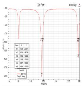
Fig.5 Modified Using U-Slot Antenna Return Loss 2.43, 3.87 GHz
