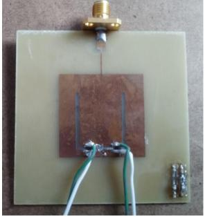
Fig.8 Experimental Measuring U-slot Antenna
