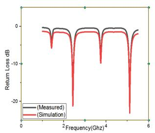
Fig.14 Proposed reconfigurable antenna return loss Simulation and Measured at 2.3,4.99GHz (Two diodes D1,D2-OFF)
