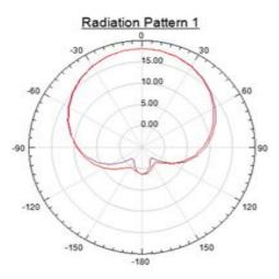
Fig.6 Modified Using U-Slot Radiation Pattern
