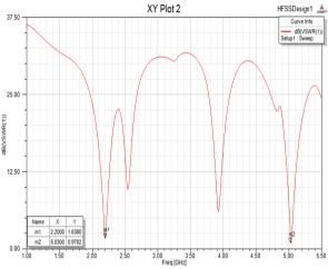
Fig.26 Proposed reconfigurable antennaVSWR 2.2, 5.3GHz (Diodes D1-OFF and D2- ON)
