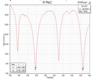
Fig.17 Proposed reconfigurable antennaVSWR 2.43 and 5.11GHz (Two diodes D1, D2-OFF)
