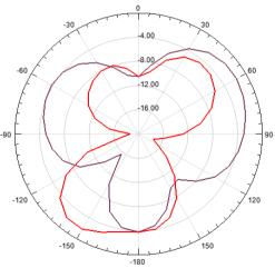
Fig.12 Proposed reconfigurable antenna Radiation pattern 4.99GHz (Both the diode D1, D2 turns ON)
