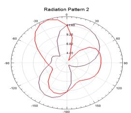
Fig.25 Proposed reconfigurable antenna Radiation pattern 5.3GHz (Diodes D1-OFF and D2- ON)
