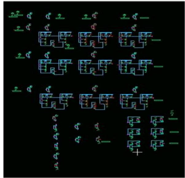
Figure 13: Braun multiplier using BKA in GDI Technology
