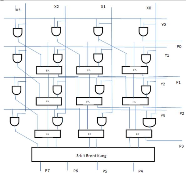
Figure6: Braun multiplier with B-K adders.
