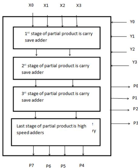
Figure4: Design structure of multiplier.
