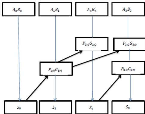
Figure 3:4 bit B-K adder.
