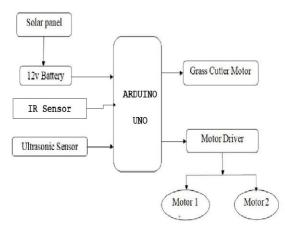
Figure 2. Block Diagram of Lawn Mower
