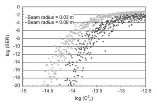
Fig.1. Typical values of BER versus different turbulent conditions characterized by Cn2 for two initial laser beam radius 0.03 and 0.09 m and laser wavelength l <sup>1</sup>/<sub>4</sub> 850 nm for a receiver at distance z <sup>1</sup>/<sub>4</sub> 1000 m. [12]
