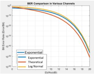
Fig.2. Simulation Of BER vs SNR for Log Normal and Negative Exponential Channel
