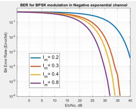
Fig. 4. BER for BPSK modulation in the Negative Exponential Channel.
