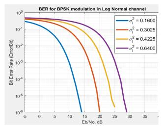
Fig. 3. The Simulated BER against the SNR in a weak atmospheric turbulence FSO channel with a scintillation  $\{\sigma^2 = 0.16, 0.30, 0.42, 0.64\}$
