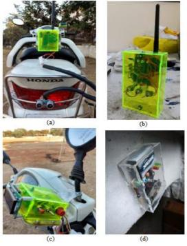
Figure 9. Fabricated and implemented (a) ZigBee Box (b) Data Center Box (c) GPS Box and (d) Collection Box
