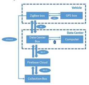
Fig. 1. Block Diagram of the SVAM System
