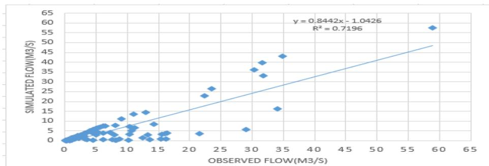
**Figure 10. Neshi station flow Validation Scattered plot**
