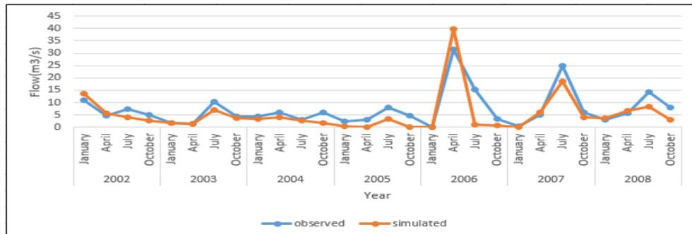
**Figure 11. Neshi station flow data during Validation**
