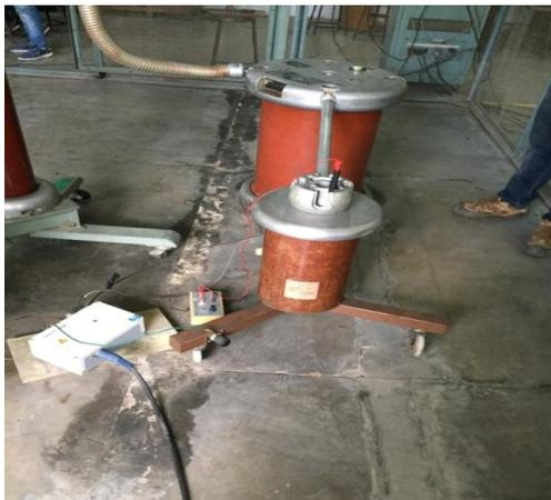
Figure 9 Discharge Capacitor and Testing Transformer
