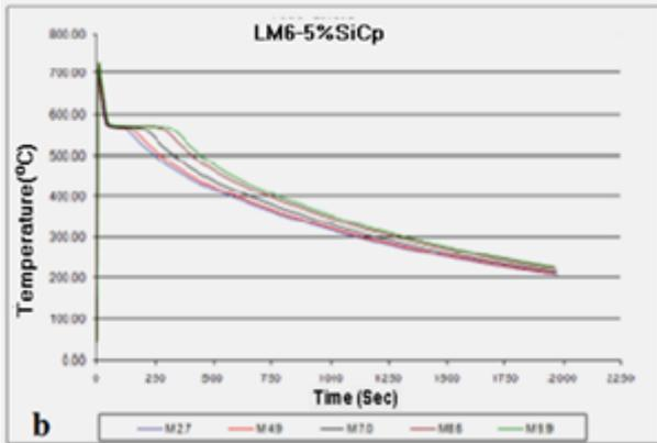
Figure 6: Cooling trends of AMMC with 5wt% SiCp at different section of casting (a) sand casting and (b) gravity die casting.
