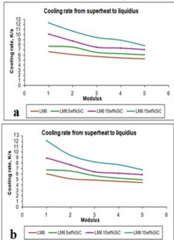
Figure 10: Cooling rates from superheat to liquidus (a) sand casting & (b) gravity die casting.
