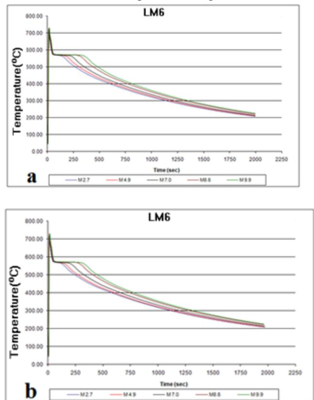
Figure 5: Cooling trends of LM6 at different section of casting (a) sand casting and (b) gravity die casting.
