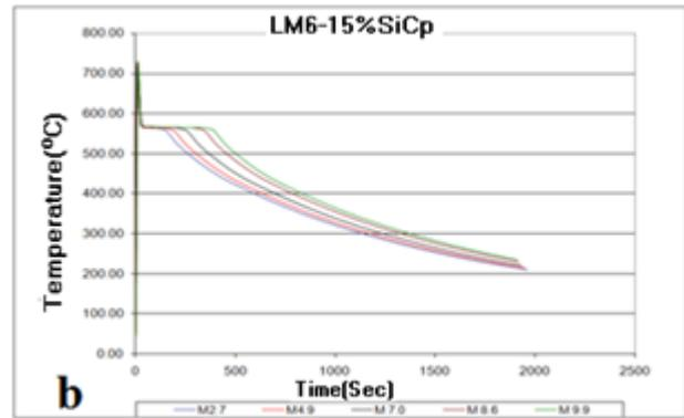
Figure 8: Cooling trends of AMMC with 15wt% SiCp at different section of casting (a) sand casting and (b) gravity die casting.
