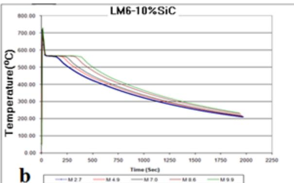
Figure 7: Cooling trends of AMMC with 10wt. % SiCp at different section of casting (a) sand casting and (b) gravity die casting.
