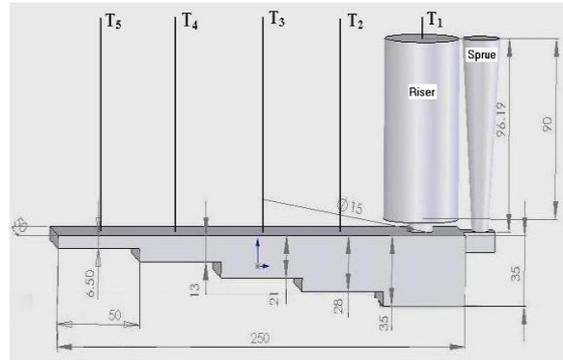
**Figure 2: The Model view and dimensions (in mm) of the mold cavity with five different thermocouples (T<sub>1</sub>, T<sub>2</sub>, T<sub>3</sub>, T<sub>4</sub> and T<sub>5</sub>).**
