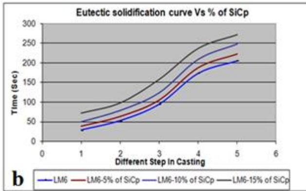
Figure 9: Effect of wt. % SiCp in eutectic solidification time at different section of casting (a) sand casting and (b) gravity die casting.
