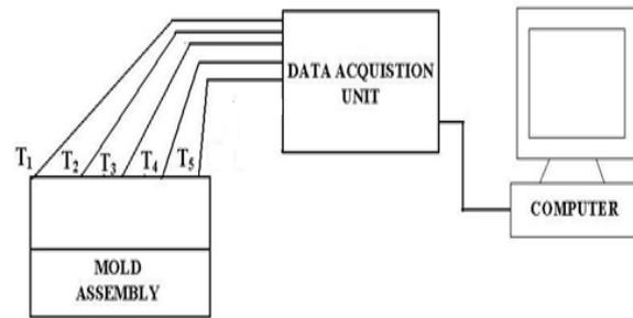
**Figure 3: Block diagram of data acquisition set-up for casting.**
