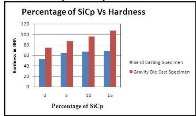
Figure 4: Hardness results by varying wt. % of SiCp.
