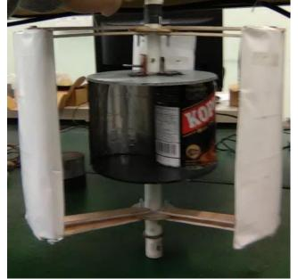
Fig. 3.Hybrid wind turbine (Savonius - Darrieus)
