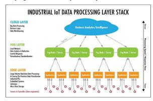
Fig 1 Layered architecture of Fog Computing
