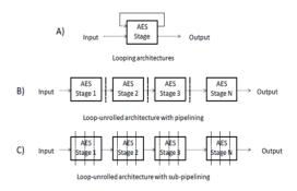
Figure.1. AES structural design
