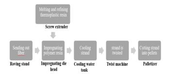
Fig. 6: Injection molding technology to produce pellet film fiber-reinforced thermoplastic composite (Tanaka, 2013)
