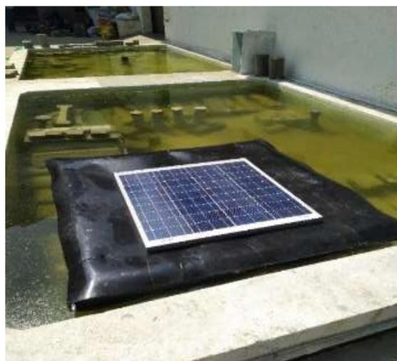
Fig 9. Floating PV panel prototype
