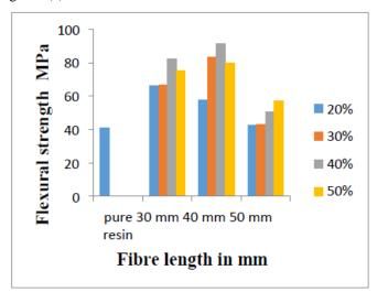
Fig. 3. Effect of fibre length on flexural strength
