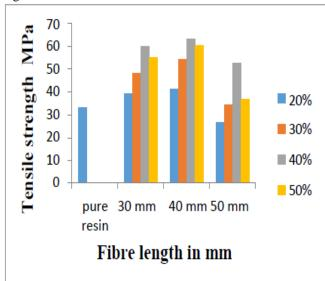
Fig. 1. Effect of fibre length on tensile strength
