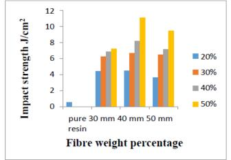
Fig. 5. Effect of fibre length on impact strength
