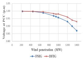
Fig. 4a. Voltage at PCC for different wind penetrations without VSC-HVDC
