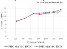
Fig. 5b. P losses for different wind penetrations with VSC-HVDC
