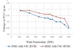
Fig. 4b. Voltages at PCC for different wind penetrations with VSC-HVDC
