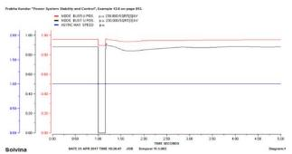
Fig. 9b. Voltage at PCC, Faulted Bus (Bus T) and Speed of wind machine - Case c
