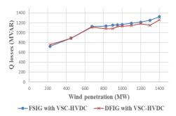
Fig. 5d. Q losses for different wind penetrations with VSC-HVDC
