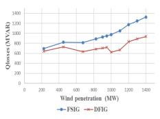
Fig. 5c. Q losses for different wind penetrations without VSC-HVDC
