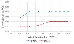
Fig.3a. Power factor at PCC for different wind penetrations without VSC-HVDC
