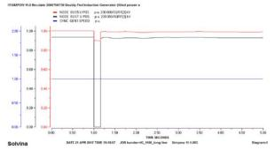
Fig. 9a. Voltage at PCC, Faulted Bus (Bus T) and Speed of wind machine - Case b
