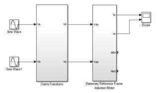
Fig. 4.Induction Motor Model in Simulink
