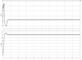
Fig. 15.Waveforms shows the motor torque Te (upper) and speed  $\omega_r$  (lower) in rad/sec. Note that if the load torque increases to 25N-m, the speed decreases slightly from 375 rad/sec to 350 rad/sec.
