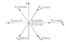
Fig. 12.Inverter switching states
