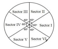
Fig. 6.Six sectors with the distinct voltage vectors
