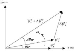
Fig. 8.Stator and Rotor space vectors
