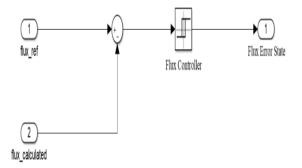
Fig. 7. Two level hysteresis flux controller
