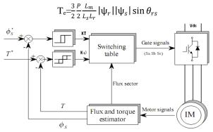
Fig. 5.DTC Block diagram with Inverter fed IM
