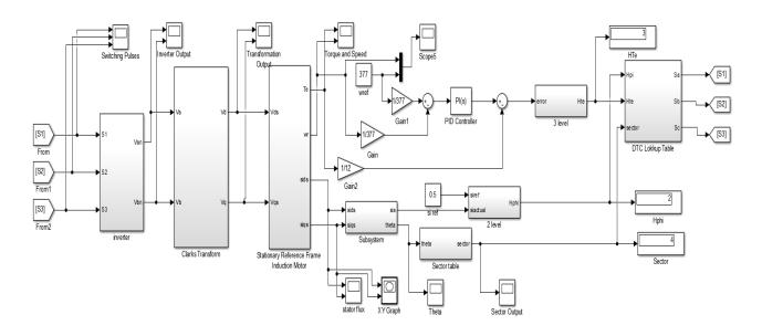
Fig. 14.Induction Motor Model with Direct Torque Control in simulink/MATLAB
