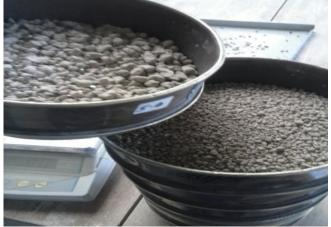
Fig 1. Sieve analysis for Aggregates Source (author 2013)
