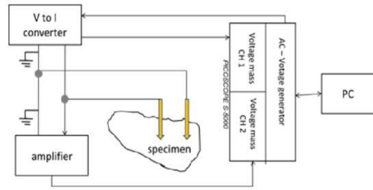
Fig. 1. The measurement setting of the electrical impedance [10].
