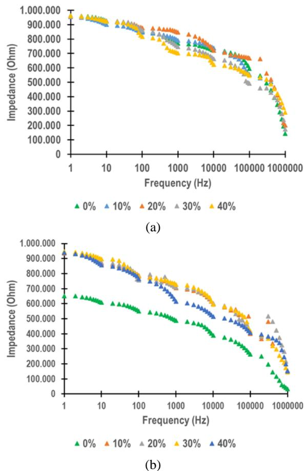
**Fig. 4. The impedance of the shrimp with formalin concentration of 10% - 40%, a) on day 1, b) on day 5.**
