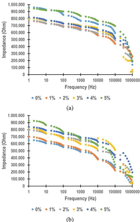
**Fig. 3. The impedance value of the shrimps with formalin 1% to 5% on a) day 1 and b) day 5**
