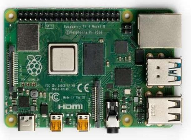
Fig 2. Raspberry pi 4 model b
