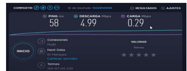
Fig. 20. Figure 19. Signal quality testing at 503 meters
