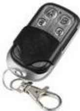
Fig. 3. Universal Control RF 433MHz [11]
