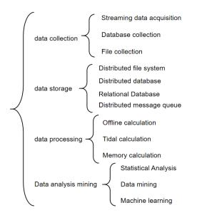
Figure 1. Smart grid big data technology structure
