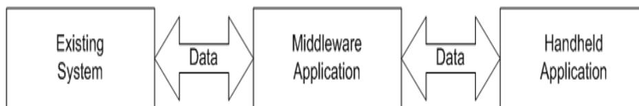
**Figure 3. Basic Mobile Architecture**
