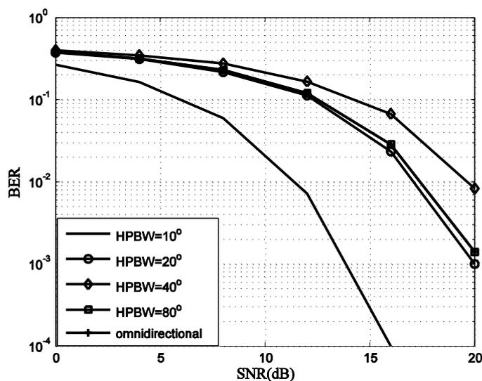
**Figure 13. BER Performance of RAKE Receiver with Different HPBW in Scenario 2**
