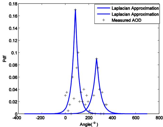
**Figure 4. Probability Density Function of AOD and Laplacian Approximation**
