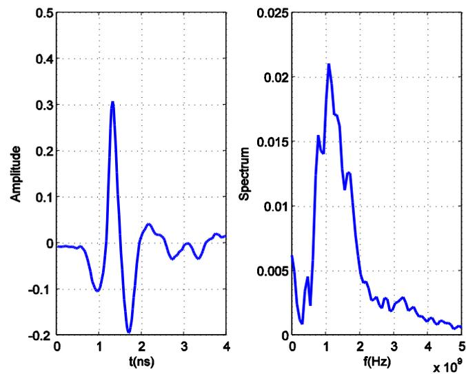
Figure 1. HL9200 Pulse Shape and Spectrum
