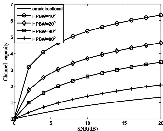
Figure 10. Channel Capacity with Different HPBW in Scenario 1
