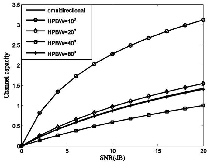
**Figure 11. Channel Capacity with Different HPBW in Scenario 2**
