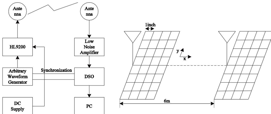
Figure 2. Diagram of System Setup and Grid for Measurement
