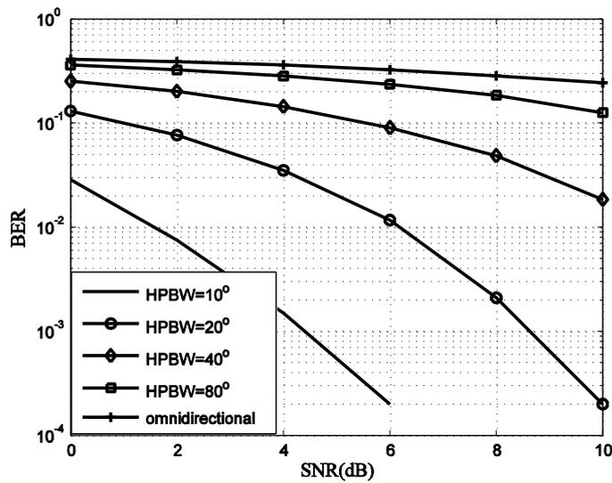
**Figure 12. BER Performance of RAKE Receiver with Different HPBW in Scenario 1**
