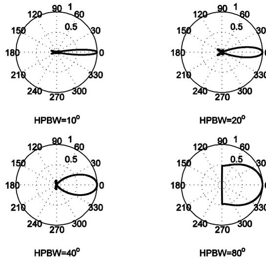
**Figure 9. Circular Horn Antenna Radiation Pattern Diagram with Different HPBWs**
