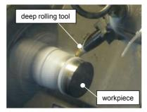
Figure 4 Experimental setup for deep rolling (see online version for colours)
