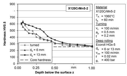
In order to improve the transformation behaviour of the special alloy X120CrMn5-2, an adaption of the preliminary heat treatment was carried out by varying the austenitising temperature  $T_A$ . Thereby, the microstructure of the material was adjusted to ensure a change in the stability of the austenite and also modified transformation behaviour.
