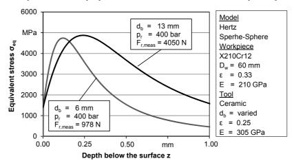
Figure 6 Equivalent stress depth profile of conventional X210Cr12 for varied process parameters
