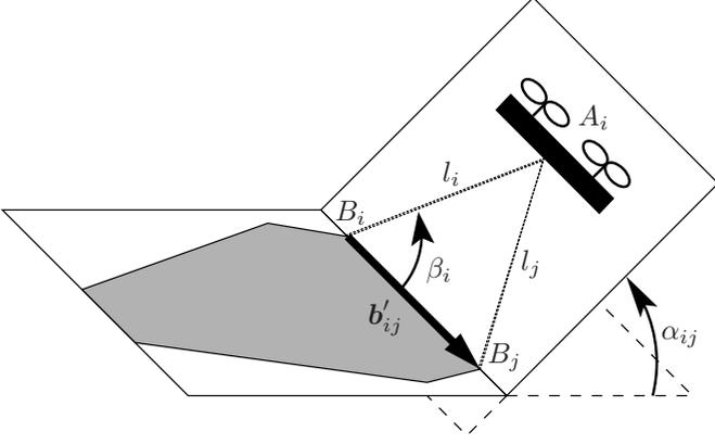
Fig. 3.  $\alpha_{ij}$  measures the angle between the plane of the platform and the plane of cables  $i$  and  $j$  attached to the same flying robot.
