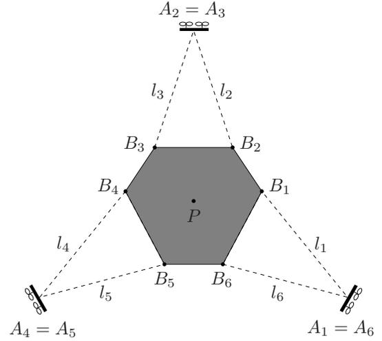
Fig. 2. Geometric structure of a generic *FlyCrane* system.
