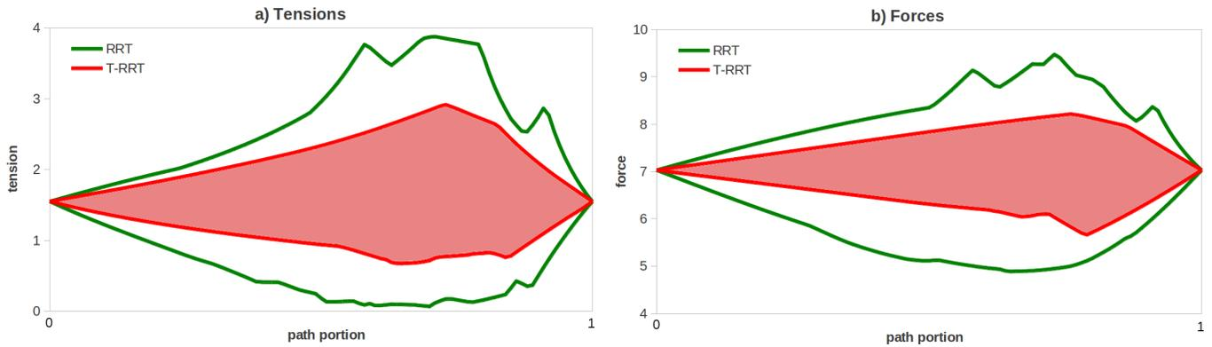
Fig. 6. Profiles of a) the tension range and b) the force range, observed over 100 paths produced by RRT and T-RRT on the *Rescue* problem. The filled areas between the red curves represent the ranges for T-RRT; the areas between the green curves represent the ranges for RRT.
