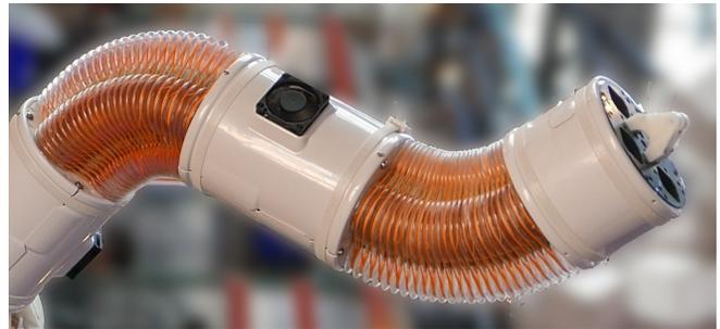
Fig. 1. Bellows-driven continuum joints are used to create robots without finite degrees of freedom. Sensing the motion of such robots is a challenge. The inductance-based sensors presented in this work will bring estimation and control to robots like the one pictured here (created by Pneubotics).
