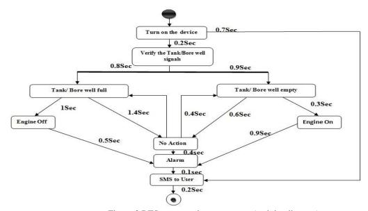
Figure.3 RTS automated water system (activity diagram)
