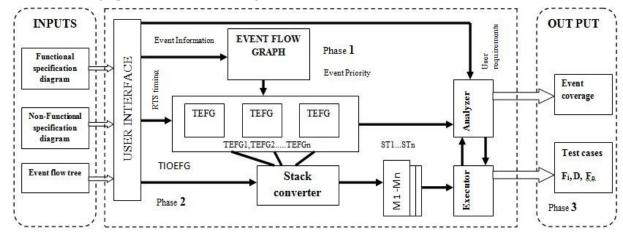
Phase1: Event flow graph converter; Phase 2: Timing event flow graph converter; Phase 3: Test case generator.
