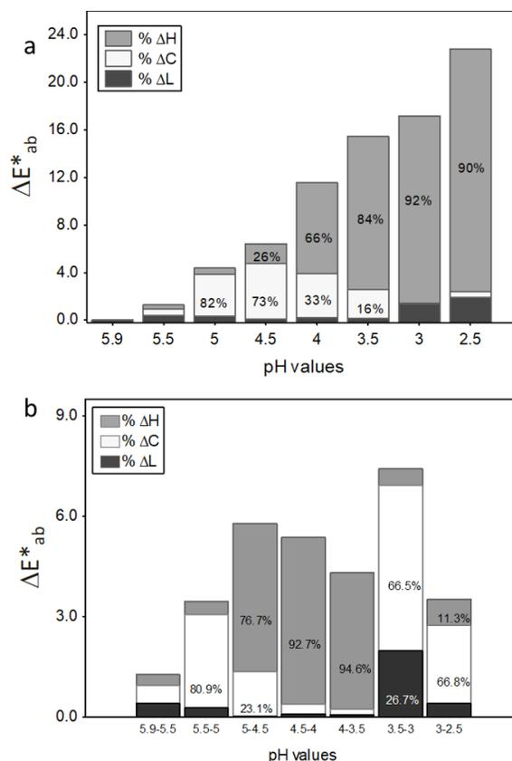
Figure 4. Color differences ( $\Delta E^*_{ab}$ ) with the quadratic variations of lightness ( $\% \Delta L$ ), chroma ( $\% \Delta C$ ), and hue ( $\% \Delta H$ ) calculated by pairs of samples as a function of pH: (a)  $\Delta E^*_{ab}$  among films at each pH (5.5-2.5) respect to natural pH (5.9), (b)  $\Delta E^*_{ab}$  among films at consecutive pH values (5.9-5.0, 5.0-4.5, 4.5-4.0, 4.0-3.5, 3.5-3.0, 3.0-2.5).
