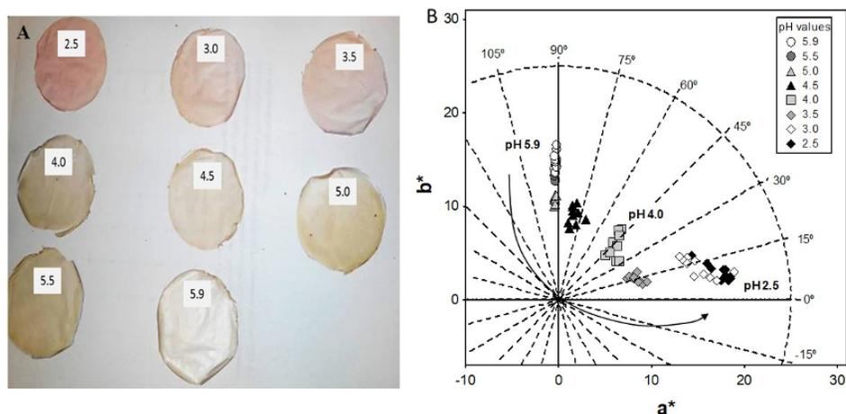
Figure 1. A) Appearance and visual color of nopal mucilage/gellan gum films enriched with red cabbage anthocyanins at different pH values (2.5-5.9), B) Evolution of the color of films within the CIELAB ( $a^*b^*$ ) diagram according to pH changes.
