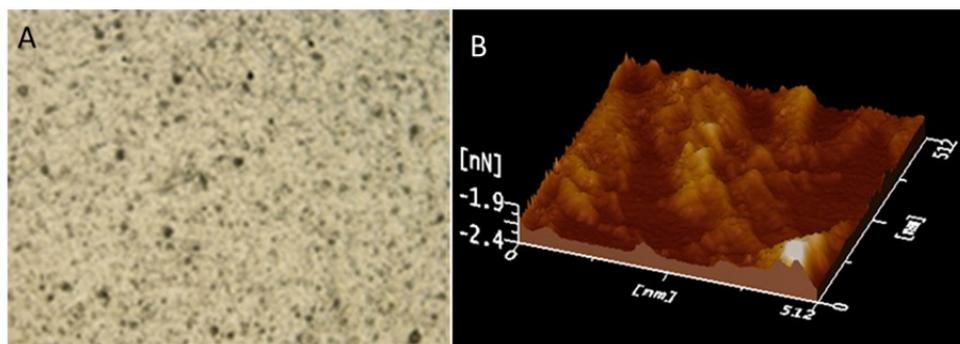
Figure 3. Micrographs of the film microstructure at natural pH (5.9): A) Optical microscopy (600x total magnification), B) Atomic force microscopy.
