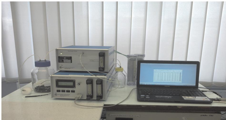
Fig. 2. The test stand for measuring biological activity – respirometer Oxymax ER-10
